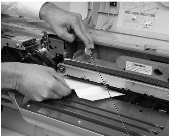
WOW® transport jam release lever
